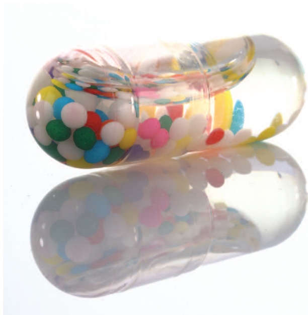
Combination fills illustrate the flexibility of soft and hard capsules. Here multiparticulates are combined with a liquid fill in a hard capsule.
