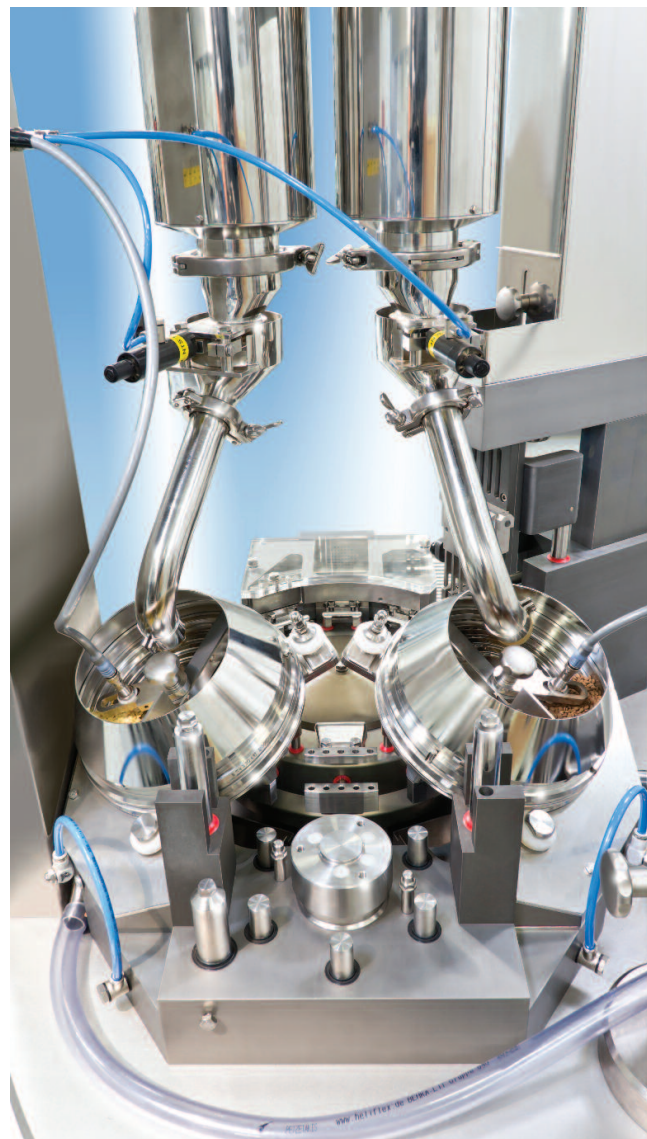
The GKF 702 from Bosch fills capsules with tablets, powders, pellets, and liquids, either individually or in combination. For powder fills, it uses either tamping pins or dosators.
